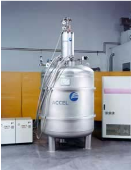
Figure 7: 2 MJ SMES developed by ACCEL (Source: ACCEL)
